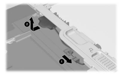
Removing the RTC Battery
